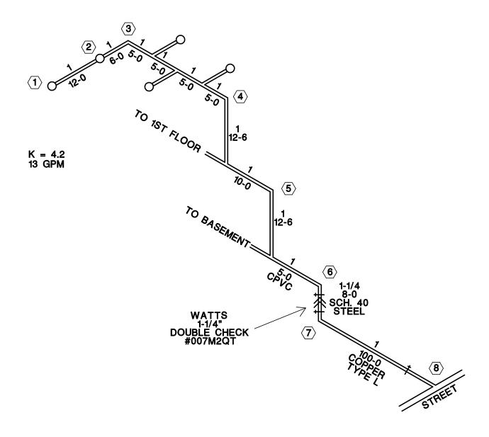
WATER SUPPLY TEST STATIC - 70 PSI RESIDUAL - 55 PSI FLOW - 100 GPM
